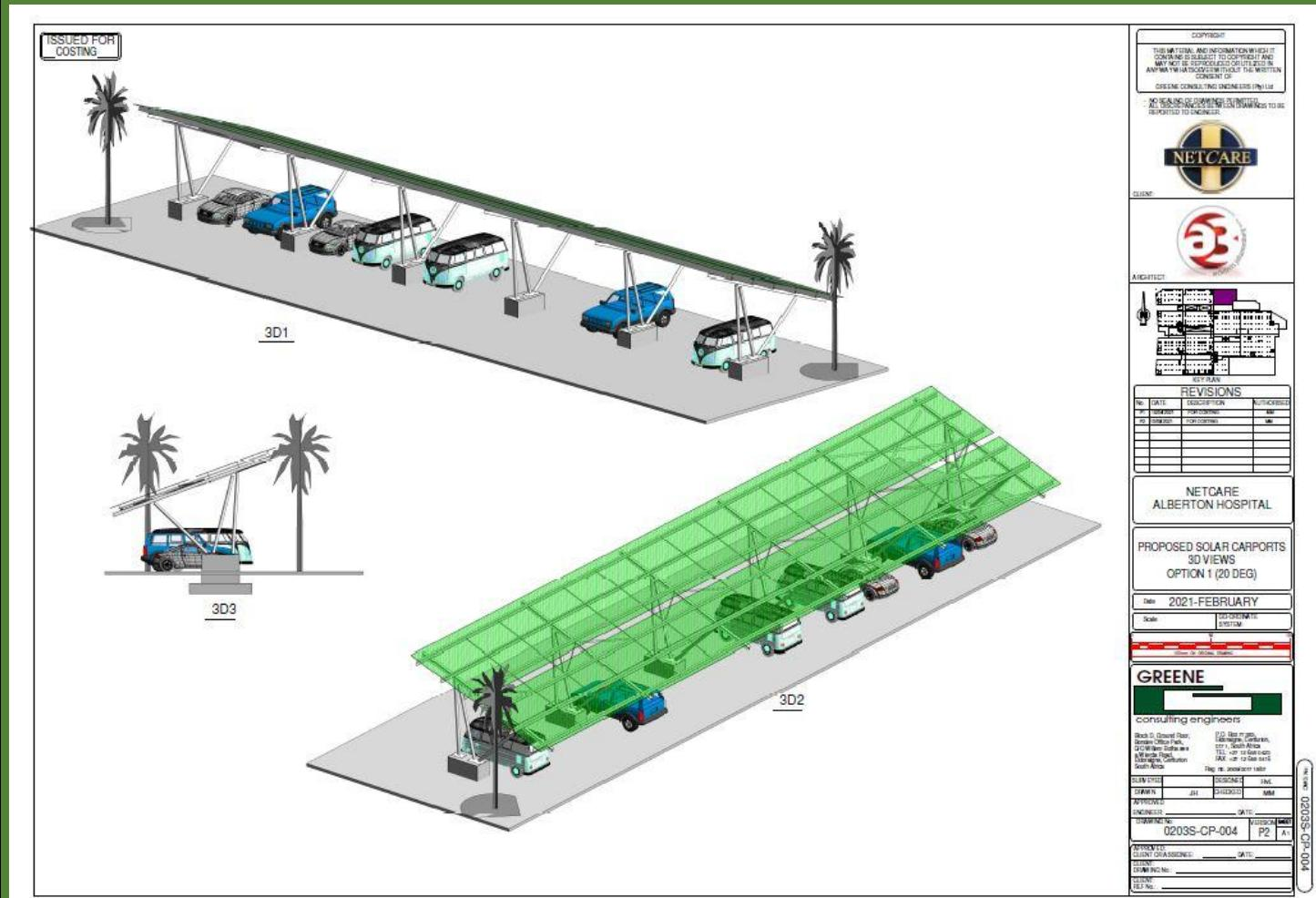
Netcare: Conceptual solar parking bays 7.5m spacing catering for three vehicles.
