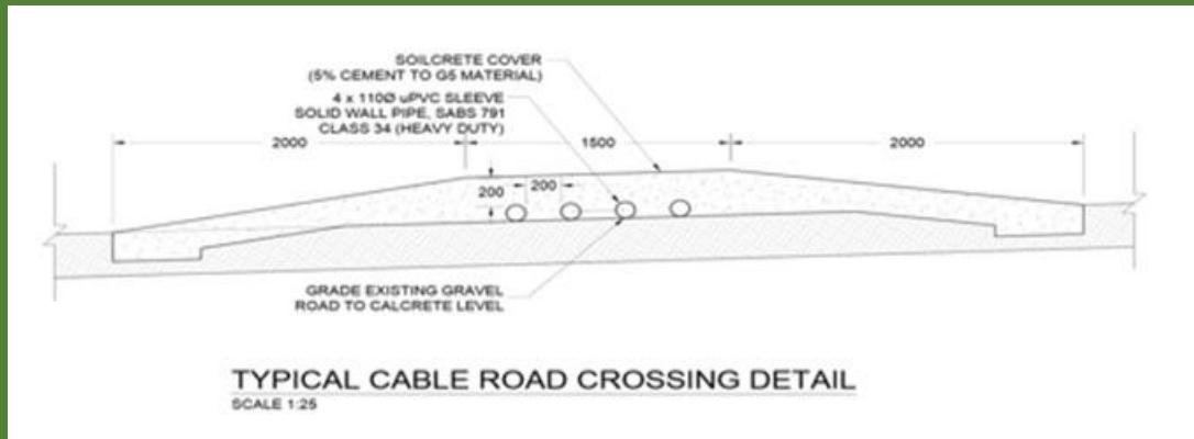
The cables will run down from the cable supports system through heavy duty uPVC sleeves that will be protected by soilcrete along the roadway.
